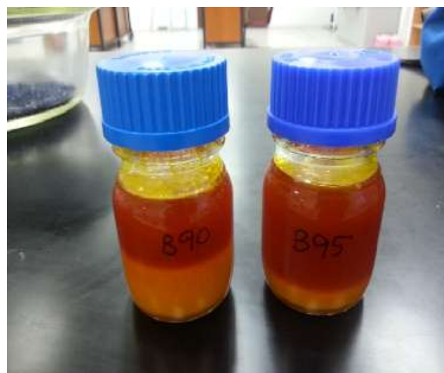
Fig. 1. Formation of emulsions observed at bottom of bottles labelled as B90 and B95 after ultrasound treatment
