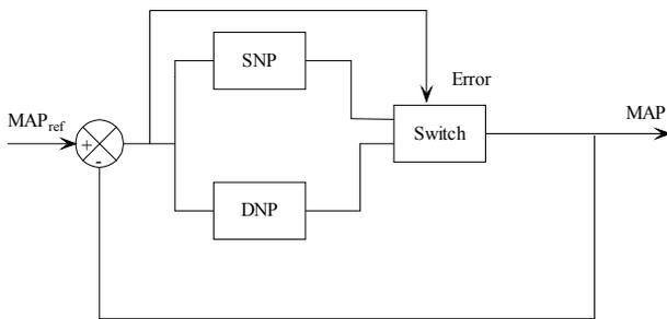
Fig.5. Switching of Controller to regulate MAP
