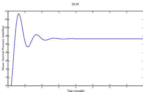
Fig.7. Z-N PI Closed loop response for infusion DP on CVS
