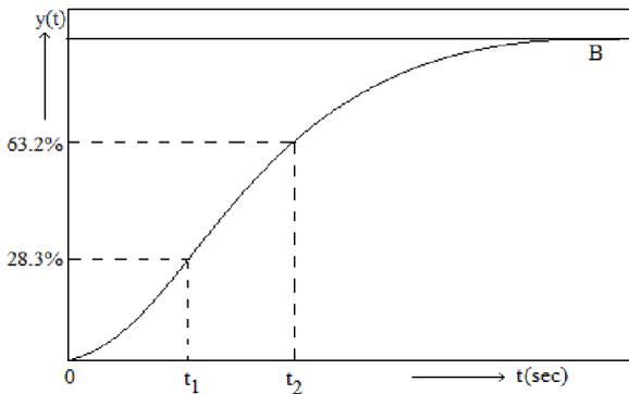
**Fig.2. Typical process reaction curve**
