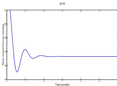
Fig.6. Z-N PI Closed loop response for infusion SNP on CVS
