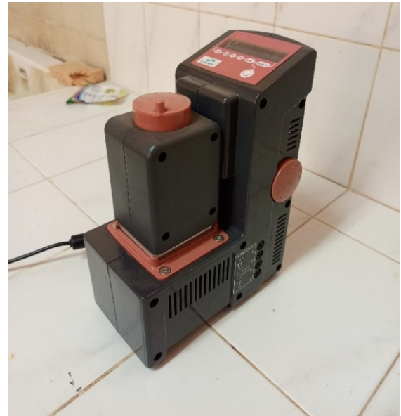
Figure 5. Thermal resistance meter (Manufacturer: Sciencéthic, Ref.005-027)
