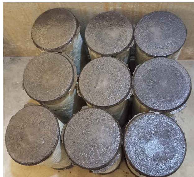
Figure 4. Concrete specimens prepared for compression testing
