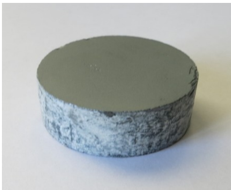
Fig.1. Photo (x1) of briquette compacted from ultradispersed \text{Si}_{0.7}\text{Ge}_{0.3}+\text{P}_{0.5} (wt.%) alloy powder at 1300°C
