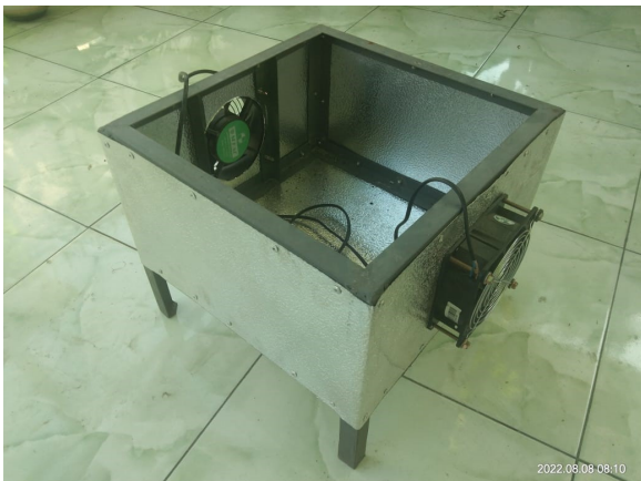
Figure 5. Blowing fans attached at the bottom sides of Vesa-2 to flow the air from the bottom to the top
