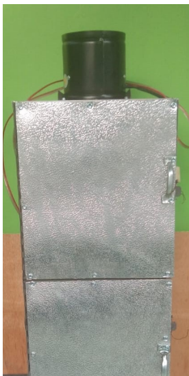
Figure 6. An inline duct fan of steel blades inhale the air from the top of Vesa-2
