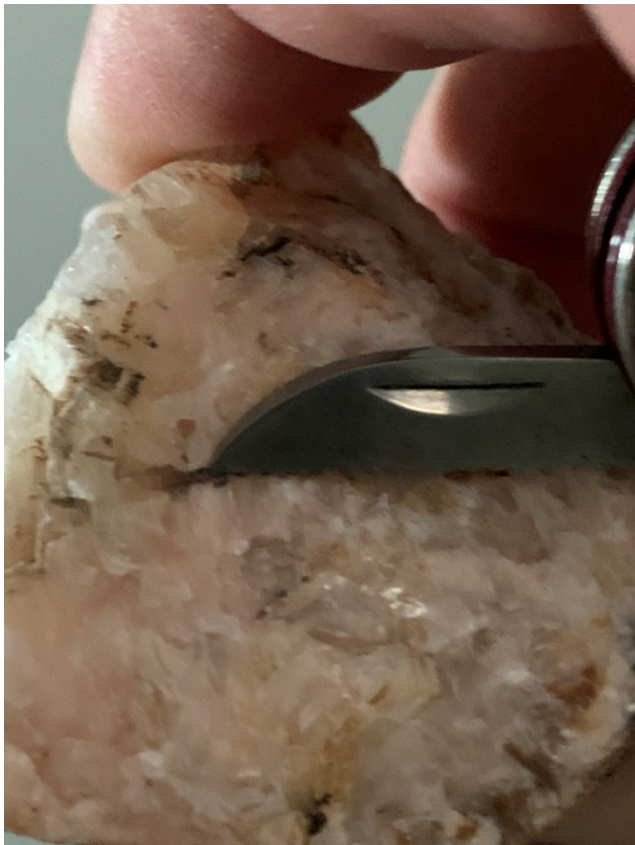
Fig. 7. Limestone and dolomite are sedimentary rocks that can be scratched with a knife: to differentiate the two, we often need to resort to the use of acids(photo by the author)
