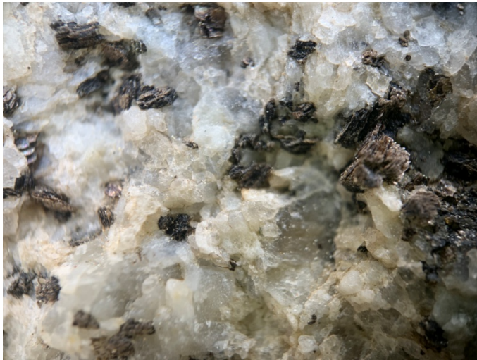
Fig. 5. The texture of the granite of an ashlar from the Monastery of El Escorial (Spain), seen with a 50X magnifying glass(photo by the author)
