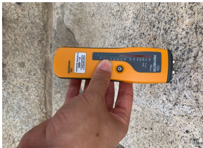
Fig. 11. Humidity measurement using a protimeter in ashlar of the facade of the Monastery of El Escorial, Spain (photograph by the author)
