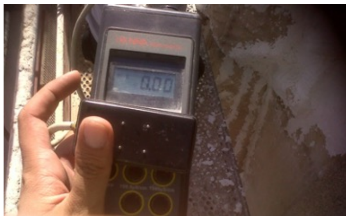
Fig. 12. Equipment used for the measurement of conductivity and, therefore, for the measurement of salts in the Patio de Santo Tomás of the University of Alcalá de Henares, in Spain (photo by author).
