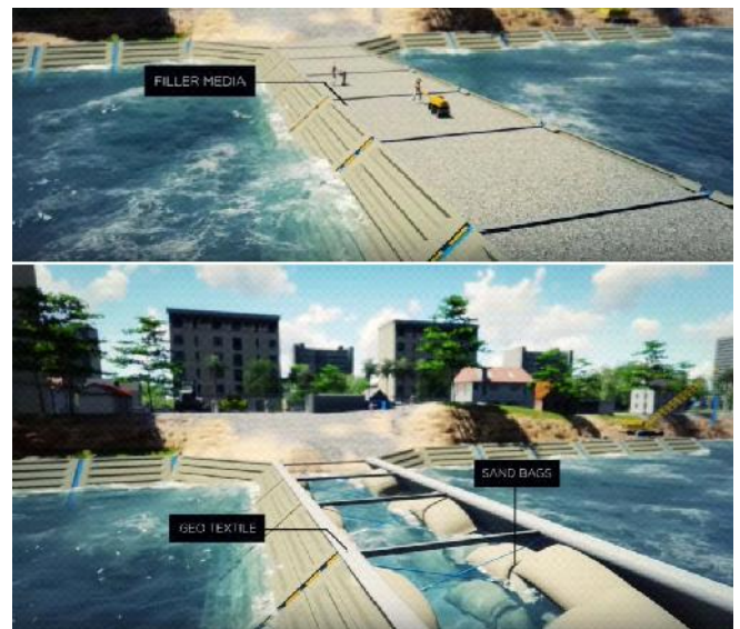
Figure 3. SPS coastal erosion protection system (Source: SPS)
