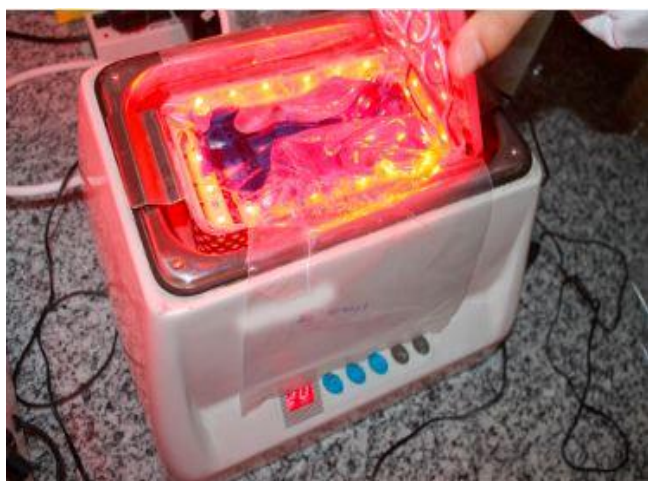
Figure 6: Photodynamic inactivation on the surface of the plates using ultrasonic Photodynamic Inactivation Device (Silva et al. , 2019).
