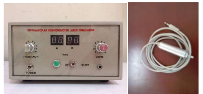
Figure 4. The intravenous low-level semiconductor laser device and the laser probe
