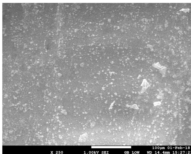
**Figure 2. FE-SEM of Torlon –Zif8(20%) mixed matrix membrane dense film**
