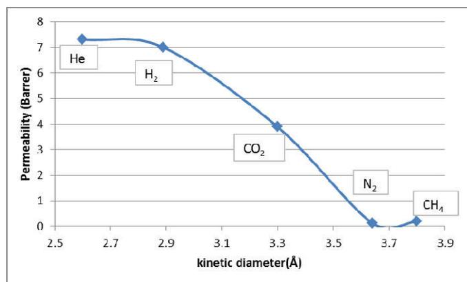
Figure 5a. Variation of gas permeability as a function of size in pure Torlon dense membrane film
