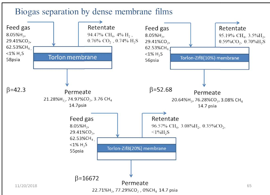
Figure 4. Results of biogas separation by Torlon, Torlon-Zif8(10%) and Torlon-Zif8(20%) dense membrane films
