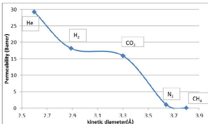
Figure 5c. Variation of gas permeability as a function of size in Torlon-Zif8 (20%) mixed matrix dense membrane film
