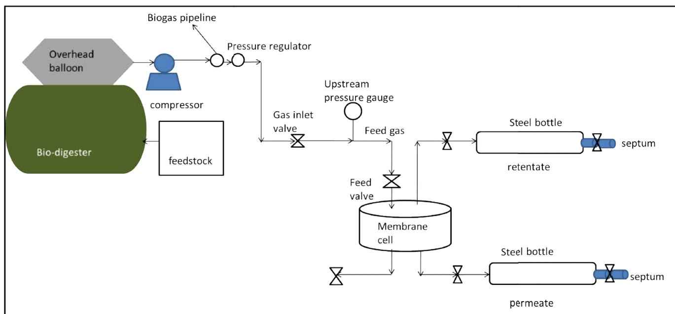
Figure 3. Schematic diagram of biogas separation by membranes
