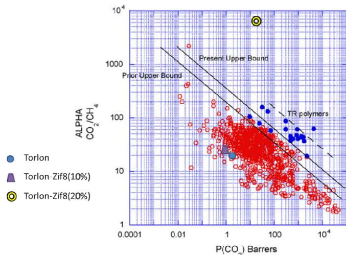
Figure 6. Gas separation performance of studied membranes on the Robeson upper bound curve for carbon dioxide-methane separation (background re-printed with permission from Elsevier)
