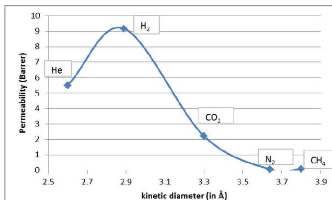
Figure 5b. Variation of gas permeability as a function of size in Torlon-Zif8(10%) mixed matrix dense membrane film
