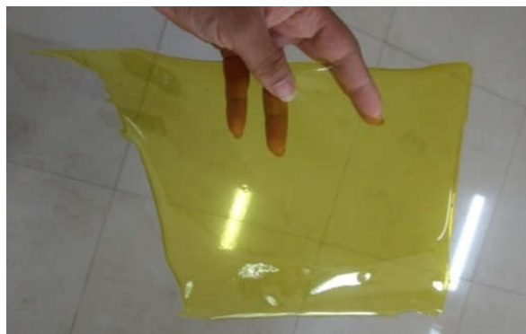
Figure 3a. Photograph of yellow Torlon AI-10 dense membrane film
