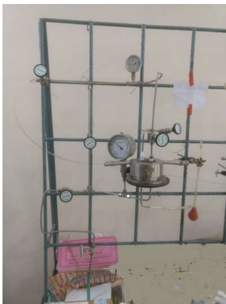
Figure 8b. Photograph of laboratory gas permeation measurement system built of Swagelok parts
