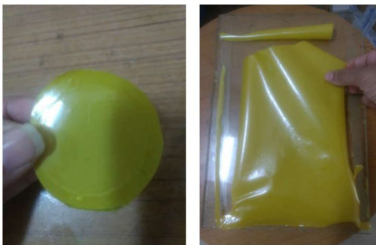
Figure 3c. Photographs of Torlon-Zif8(20%) mixed matrix dense membrane films
