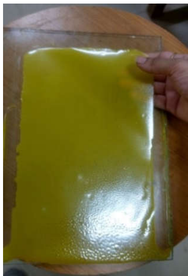
Figure 3b. Photograph of Torlon-Zif8(10%) mixed matrix membrane dense film
