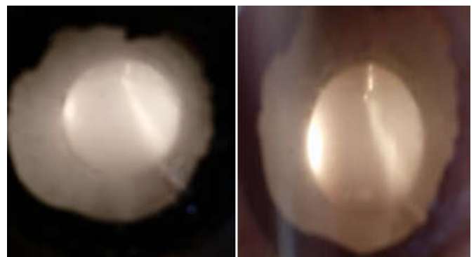
Fig. 3. Spray image at 8bar as chamber pressure for POME and Diesel
