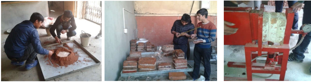
Figure 2. Preparation of Surkhi mortar
