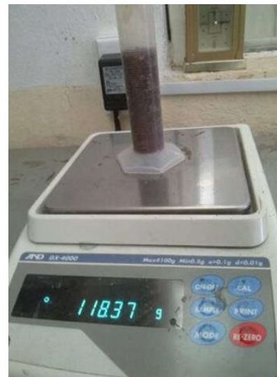
Figure 4. Weight of water and natural gap material in the volume occupied by the material
