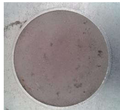
Figure 2. Gap material with unstable clay land within a consolidation ring
