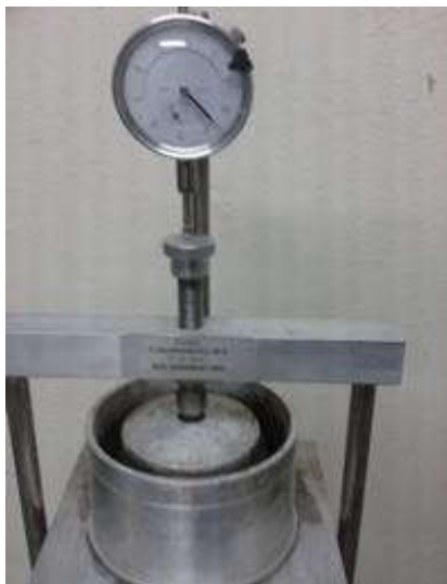
Figure 3. Growth test for unstable clay land with natural material
