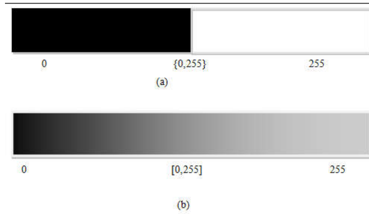
Figure 1: Representation of (a) Salt & Pepper Noise with R_{i,j} \in \{nmin, nmax\} , (b) Random Valued Impulsive Noise with R_{i,j} \in [nmin, nmax]
