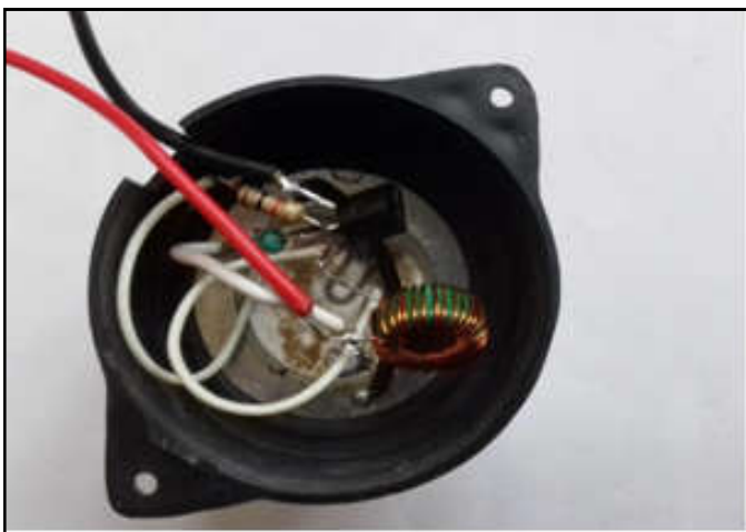
Figure 9. An electric buzzer alarm
