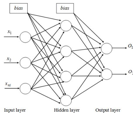
**Fig. 2. Architecture of feed forward neural network**
