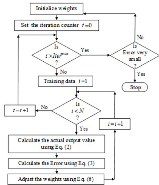
Fig. 3 Flowchart of the backpropagation learning algorithm
