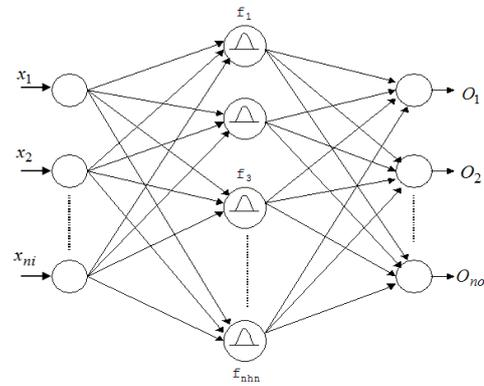
Fig. 4. Structure of Radial Basis Function Network
