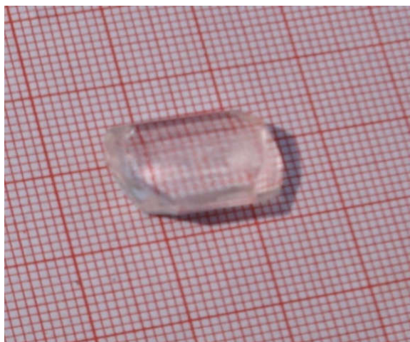
Figure 2. Pure TGS crystal
