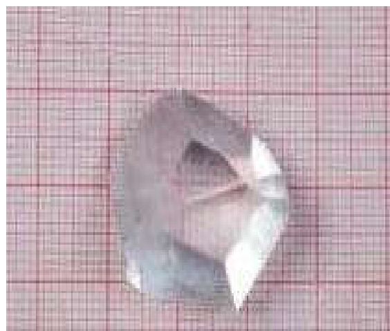
Figure 3. TGS crystal admixed with Perchloric acid (30 mole %)
