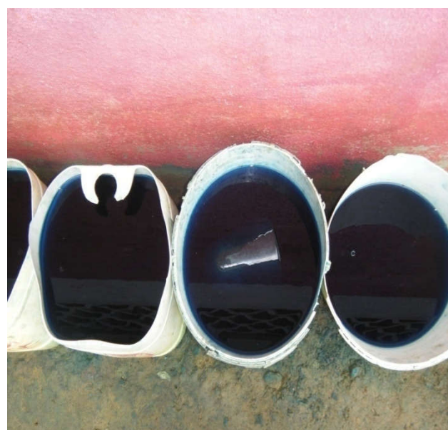
Figure 2. Acid and rain water solution colored in dark blue with Iragon
