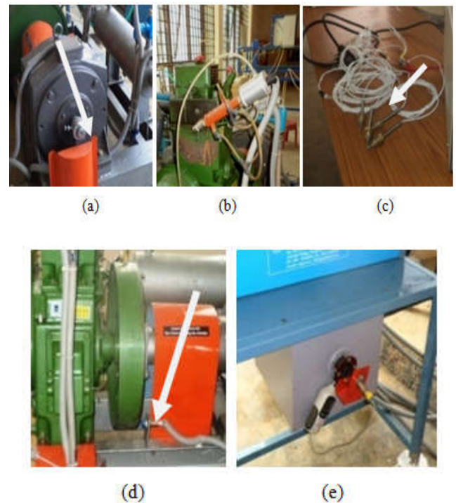
Fig. 3. The different sensors used for the measurements a) Piezoelectric pressure sensor b) RTD Temperature sensor c) Proximity speed sensor d) Strain gauge load cell based torque sensor and e) Velocity sensor.
