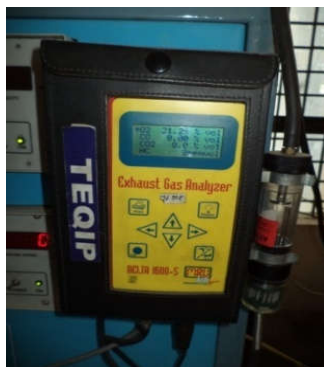
Fig. 4. Flue gas analyzer
