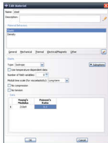
Fig. 4.5. Entering the steel element properties in ABAQUS
