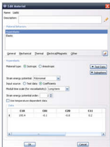
Fig. 4.4. Feeding ABAQUS with the coefficients and constants of strain energy functions for modeling rubber elements
