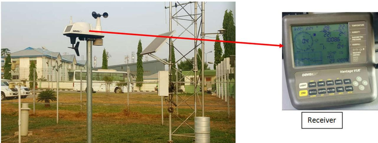
**Figure 3. An Automatic weather station at the Abuja international Airport with sensors which measure pressure, wind speed and direction, dew point and humidity and displays the data/ weather information on the receiver to the right of the enclosure**
