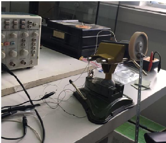
Fig. 21. Set up for the resolver
