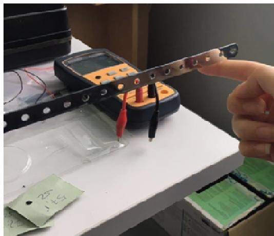
Fig. 22. Using the resolver and measuring the accuracy
