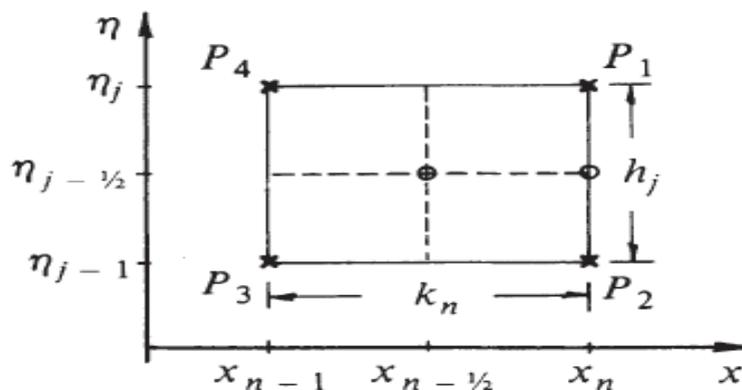
**Figure 1. Finite difference grid for the Box Method**
