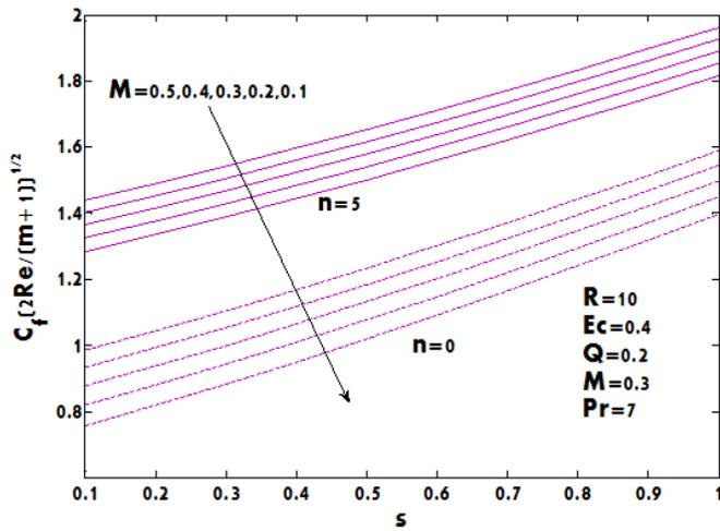
Figure 8. Effects of magnetic field parameter  $M$ , power index parameter  $n$  and suction/injection parameter  $s$  on skin friction coefficient
