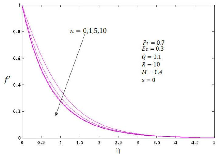
Figure 3. Effect of power index parameter  $n$  on velocity profile
