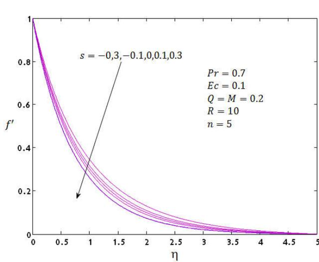
Figure 4. Effect of suction/injection parameter  $s$  on velocity of the fluid
