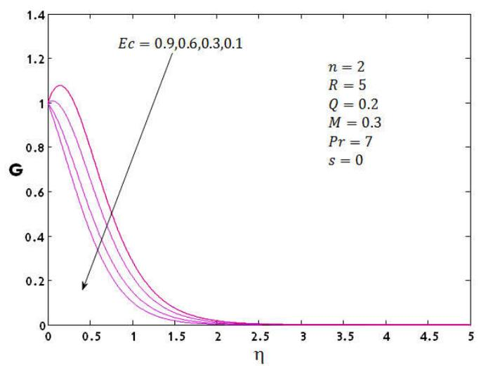
Figure 7. Effect of Eckert number  $Ec$  on temperature of the fluid
