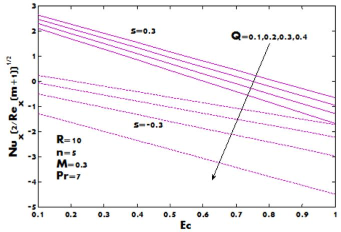
Figure 9. Effects of heat source/sink parameter  $Q$ , Eckert number  $Ec$  and suction/injection parameter  $s$  on surface heat transfer rate
