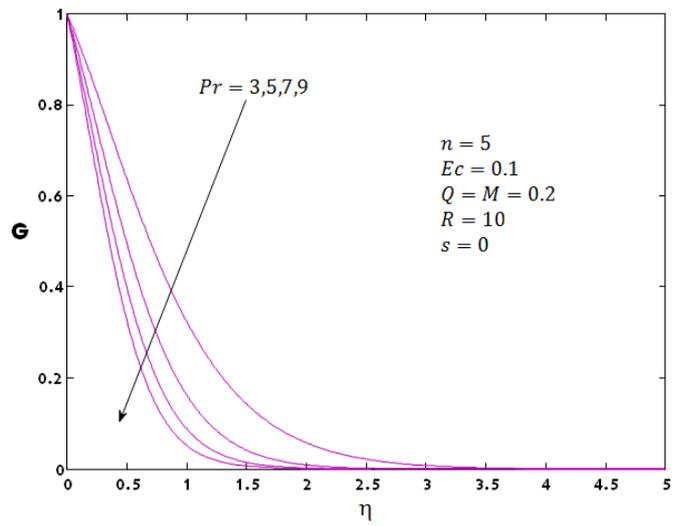
Figure 5. Effect of Prandtl number  $Pr$  on temperature
