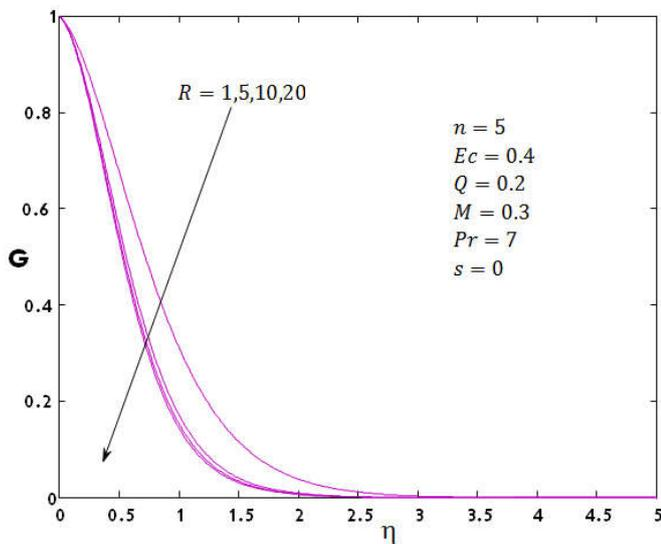
Figure 6. The effect of radiation parameter  $R$  on temperature of the fluid
