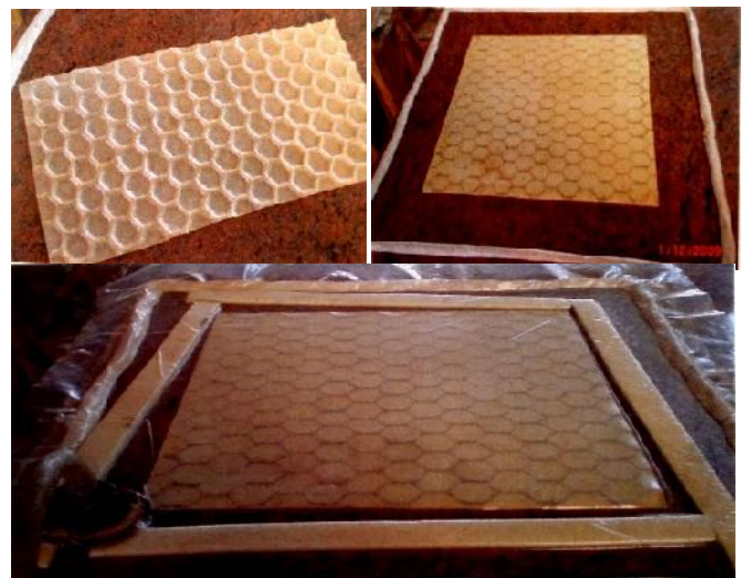
Figure 4. Fabrication of honeycomb sandwich panel
