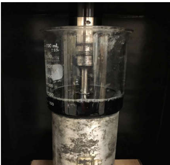
Figure 3. Sonicator Setup for nanoparticle Dispersion
