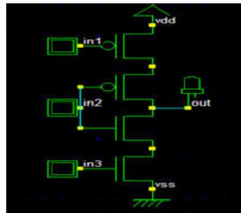
Fig. 1. Sleep transistor approach
