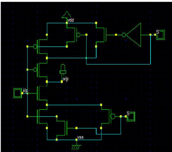
Fig. 6. Variable Body Biasing
