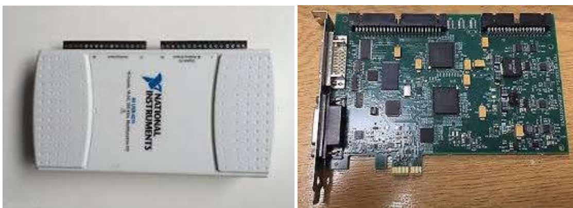
Figure 7. Data Acquisition Hardware (DAQ, NI USB-6211)
