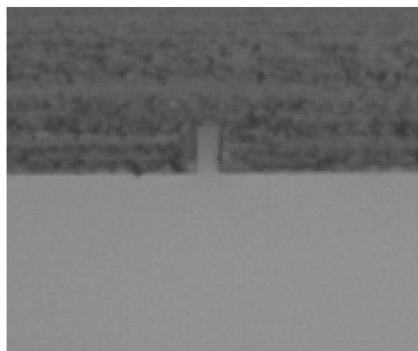
Figure 2. Cross sectional area of a PDMS microfluidic channel
