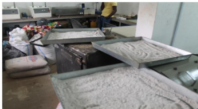
**Fig. 1. Drying of RHA from different locations in the Laboratory before analysis**
