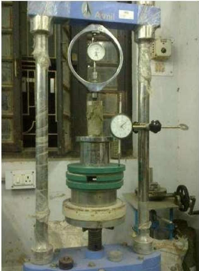
Photographic image showing test setup of UCS
