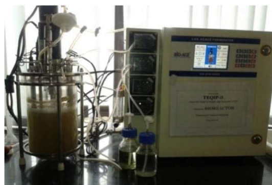
Figure 2. Photograph of lab fermenter with digital display to monitor the bioprocess
