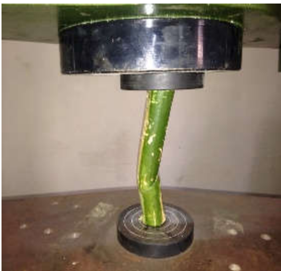
Figure 2. Bamboo strut in UTM
