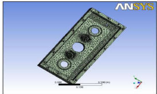
Fig : Meshed Gear housing
