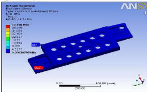
Fig : Von-Mises stress in Spindle housing
