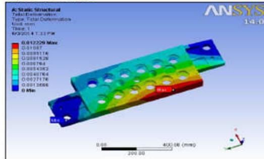
Fig : Total deformation of Spindle housing
