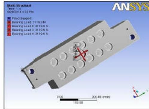
Fig : Bearing load on spindle housing
