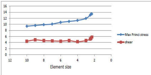
Fig. Graph of maximum Principal Stress and shear stress v/s element size
