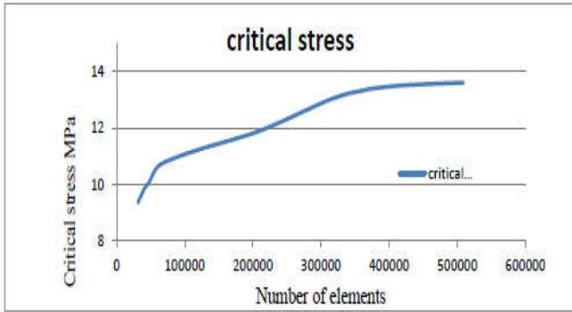
Fig. Graph of Critical Stresses v/s number of elements
