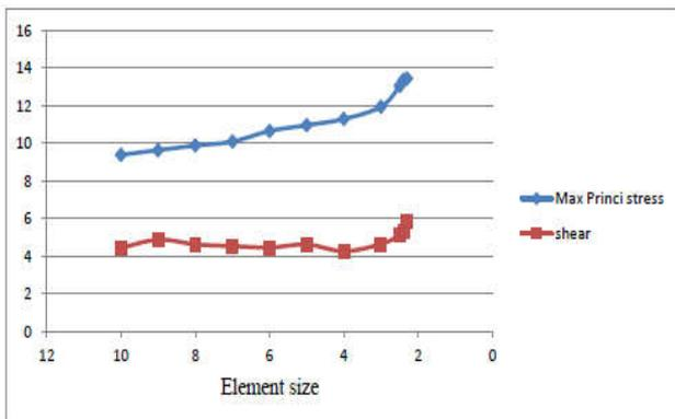
Fig. Graph of Max principal stress and shear stress v/s element size
