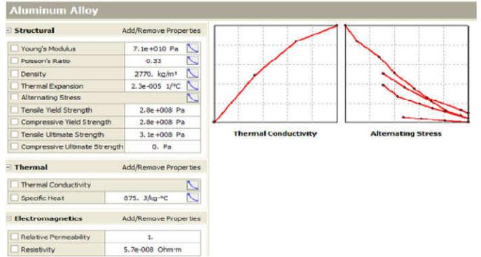
Fig. Material properties of Aluminum alloy
