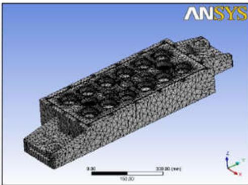
Fig. Meshed spindle housing
