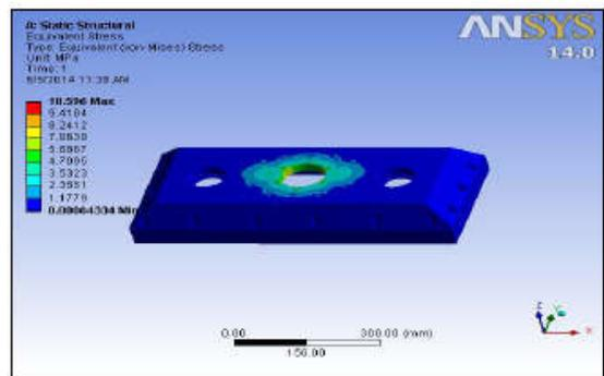
Fig: Von-Mises stress in Gear housing
