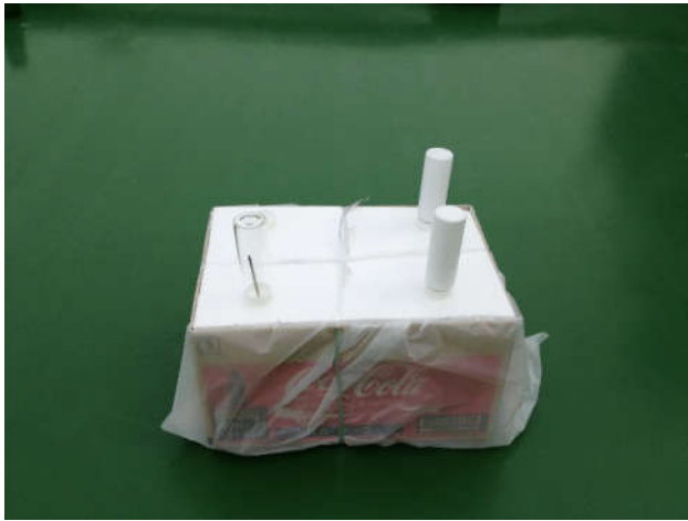
Fig. 3. Photograph of apparatus used for measuring temperatures in glass bottles outdoors
