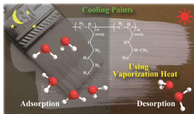
Fig. 2. Graphical abstract of this study. Water molecules are adsorbed on NIPAAm-co-BA in night and desorbed on hot daytime. By the vaporization heat of water, rooms can be cooled. This system can actuate without any electric energy and or labors
