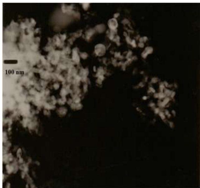
Fig 10. TEM sets nano-crystalline (particles 20-100 nm) HA cc.
