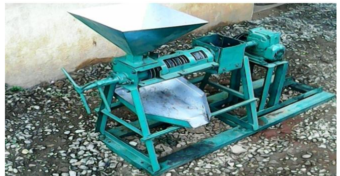
Fig. 2. Picture of the Soya Bean Oil Extracting Machine
