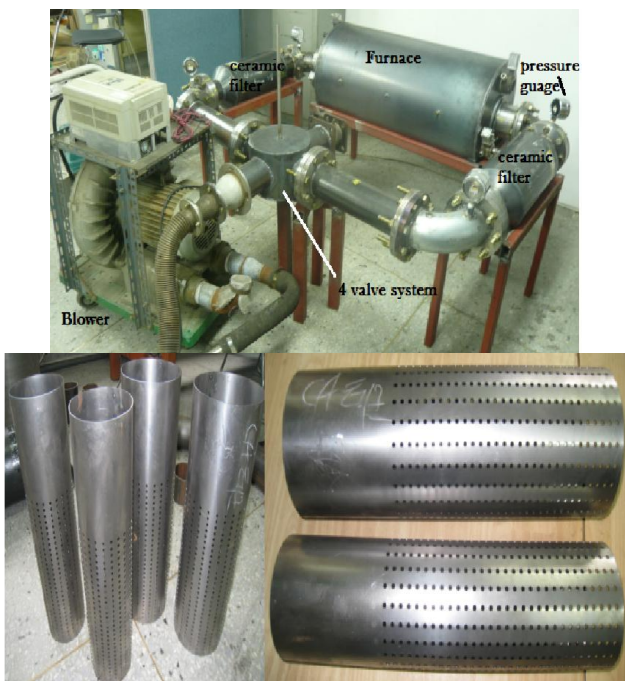
Fig. 1. Regenerative burner and testing air-distributors
