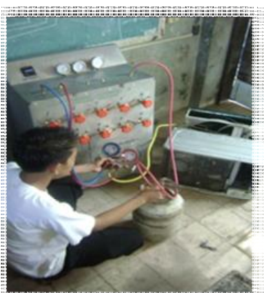
Figure 8. MRRM on Recovery Process
