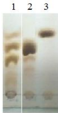
Figure 8. Thin-layer chromatography analysis of the main hydrolysis products of corn raw starch by the purified \alpha -amylase
