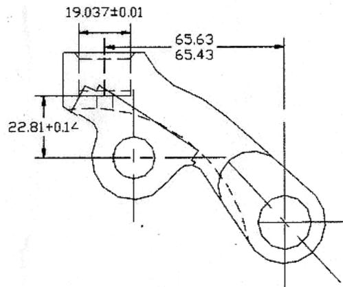
Fig. 6. Socket bore drilling
