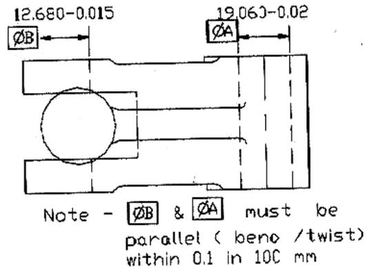
Fig. 5. pin hole boring
