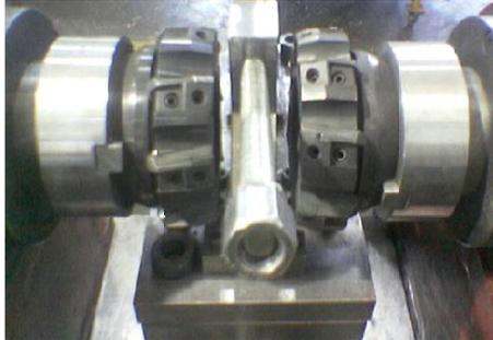
**Fig. 8. Duplex milling machine**
