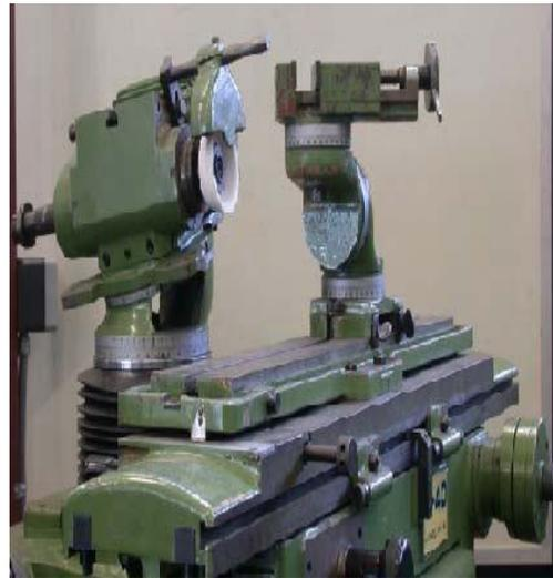
Fig. 16. Tool and cutter grinder
